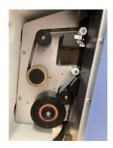
2. Feed the ribbon through the instrument ensuring that the ribbon is fitted in the correct position over every spool.
